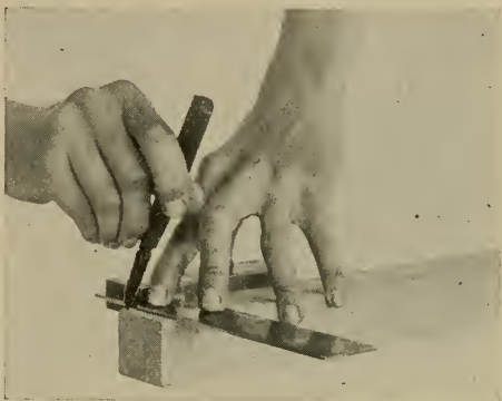
Fig. 65—Setting Try-square at Corner
